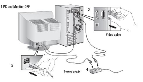
**NOTE** The location of your PC's video outlet may be different to the one shown in the diagram. Refer to the manual that came with your PC, if necessary.
